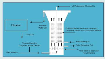
Actina™ Enhanced combines coagulation with hardness and metal precipitation into one process step that maximizes performance, reduces overall operating costs and can eliminate the need for a separate pre-treatment technology.
